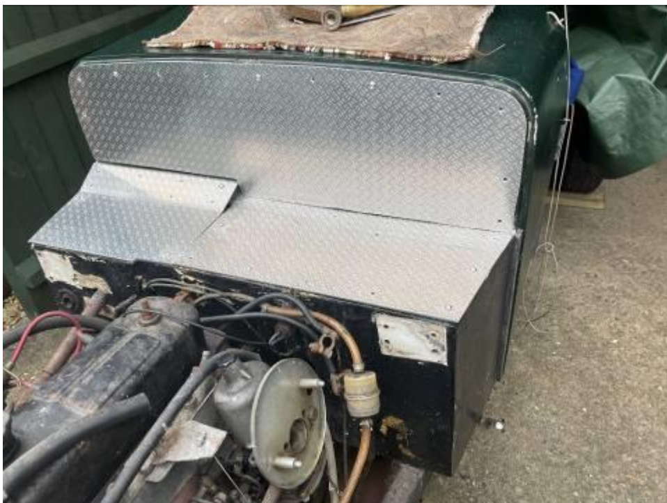
Trial fitment of the completed panels.
