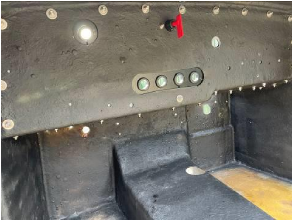
Note that the cut-outs in the fibreglass allow the grommets to fit in the chequer plate only.
